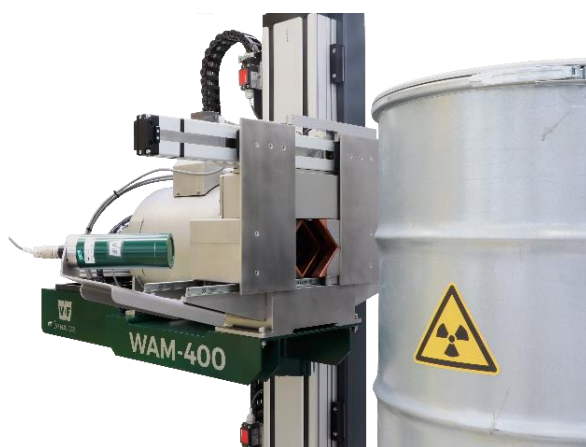
Collimator with an adjustable aperture and the MDG-12S detector for the Fast-Scan function
